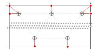
(4) The effective area to be injected when arranging grouting holes in a matrix is shown in the following figure:
