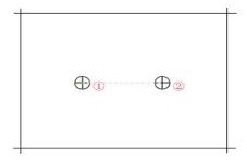
(2) The grouting holes are arranged in a linear manner, which is suitable for the leakage grouting of the long and thin belt parts.
