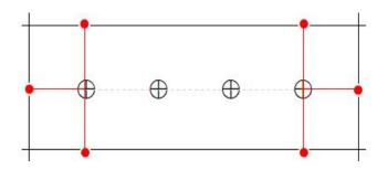
(3) The effective area to be injected when grouting holes are arranged crosswise along both sides of the crack is shown in the following figure:
