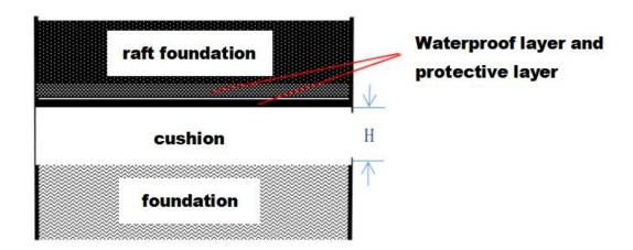
In theory, the maximum volume of the cavity to be grouted is equal to the volume of the whole cushion, which is expressed by formula (1):
