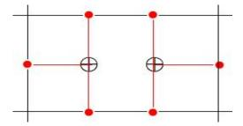
(2) The effective area to be injected when the grouting holes are arranged in a linear manner is shown in the following figure:
