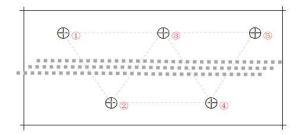
(4) The grouting holes are arranged in a matrix shape, which is suitable for grouting in discontinuous flaky leakage areas.
