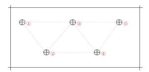
(5) Plum shaped grouting holes are suitable for large area or overall leakage grouting.
