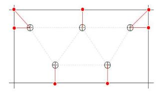
(5) The effective waiting area for grouting holes arranged in quincunx shape is shown in the following figure:
